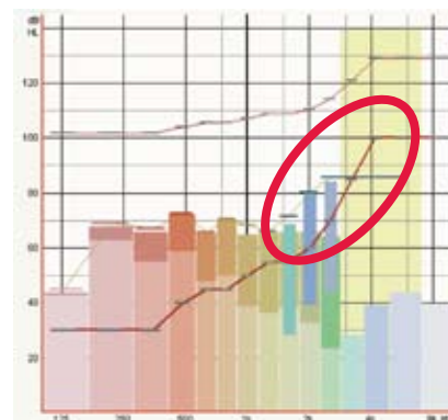
Figure 6: Conversational Speech in AE program. NOTE: The Audibility Extender provides more information (audibility) along the slope of the audiogram. The frequencies that are inaudible with the Master program are now audible.
