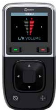
Fig. 4. With the M-DEX it is possible to change volume separately in the left and right ear.
