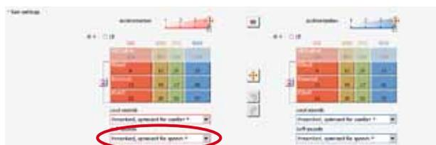
Fig. 3. It is not recommended to change the mode for soft sounds. Instead, adjustment of gain for soft sounds should be restricted to the specific frequency region where feedback occurs.
