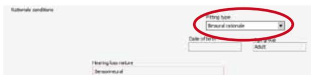
Fig. 5. The fitting rationale must be changed from Monaural to Binaural if a pair of SUPER hearing aids are fitted individually in Compass.
